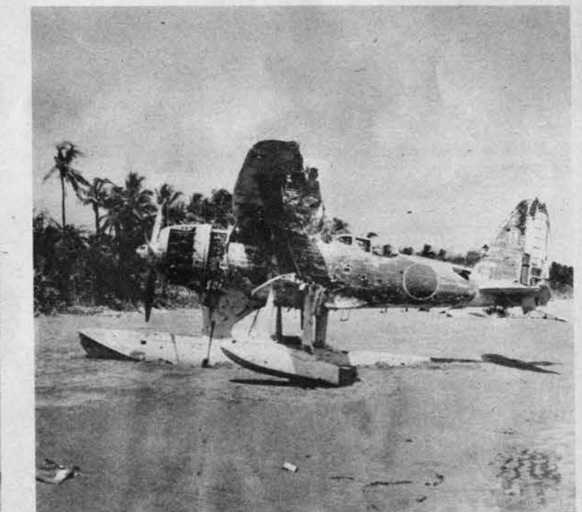
Staggered wings and wingtip floats help to identify Pete. Armament consists of two fixed 7.7-mm. machine guns firing forward and single flexible 7.7 in rear cockpit. Pete replaced an earlier float biplane, Dave.
